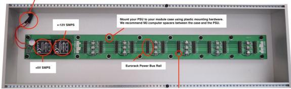
This is the -12V header pin. Connect the eurorack power bus cable in the correct orientation, with the red line positioned at the bottom of the header pins. Failure to do so may result in damage to your PSU and eurorack module(s).
