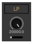
This low-pass filter is modeled after an analog low-pass resonating filter. There is a resonance control slider underneath the filter frequency cutoff knob in a similar fashion to the high-pass filter on the front end of the signal chain. This filter is ideally placed in the in-series signal chain to tame and sculpt your unwieldy distorted textures.
