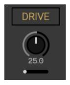
Drive is an amplitude dependent distortion module. You can increase the drive amount by increasing the drive knob towards a value of 100. A value of 0 will not apply any additional gain or soft/hard clip distortion to your signal. You can crossfade between soft and hard clip distortion using the horizontal slider underneath the drive knob.
