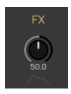
This is a Dry/Wet control, which regulates the proportion of processed to unprocessed sound. Adjustments to the FX knob do not affect signal processing, as this is done exclusively by the other modules.
