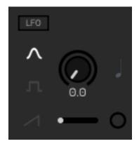
Each module has its own dedicated Low Frequency Oscillator (LFO). Each LFO can be turned on by clicking the small button located in the top-left corner and has its own dedicated amount slider located next to the LFO Speed slider. You can choose from sine, square and saw waveform types.
