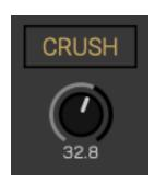
Crush allows you to quantize your incoming signal to emulate a classic bit crushing effect. Both depth and rate are tied to one single knob and scaled in such a way to leverage this kind of distortion synthesis as best as possible. Try combining this module by changing your oversampling factor using your automation lanes.
